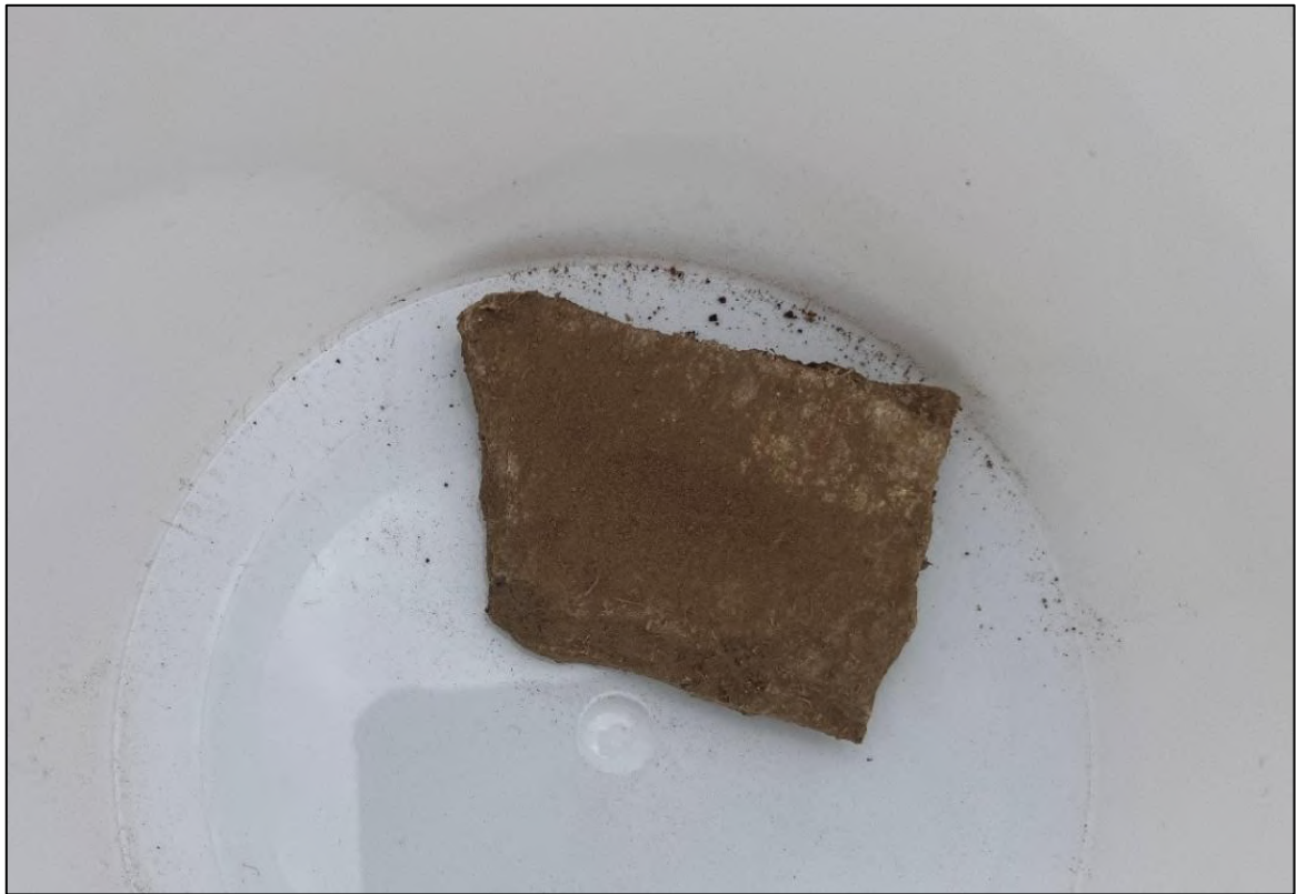
Figure 3-E: Confirmed chrysotile cement in SL11
