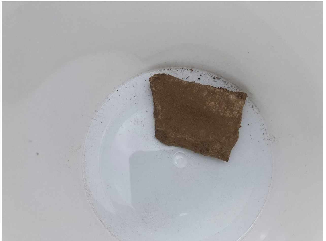
SL11 – Confirmed chrysotile cement
