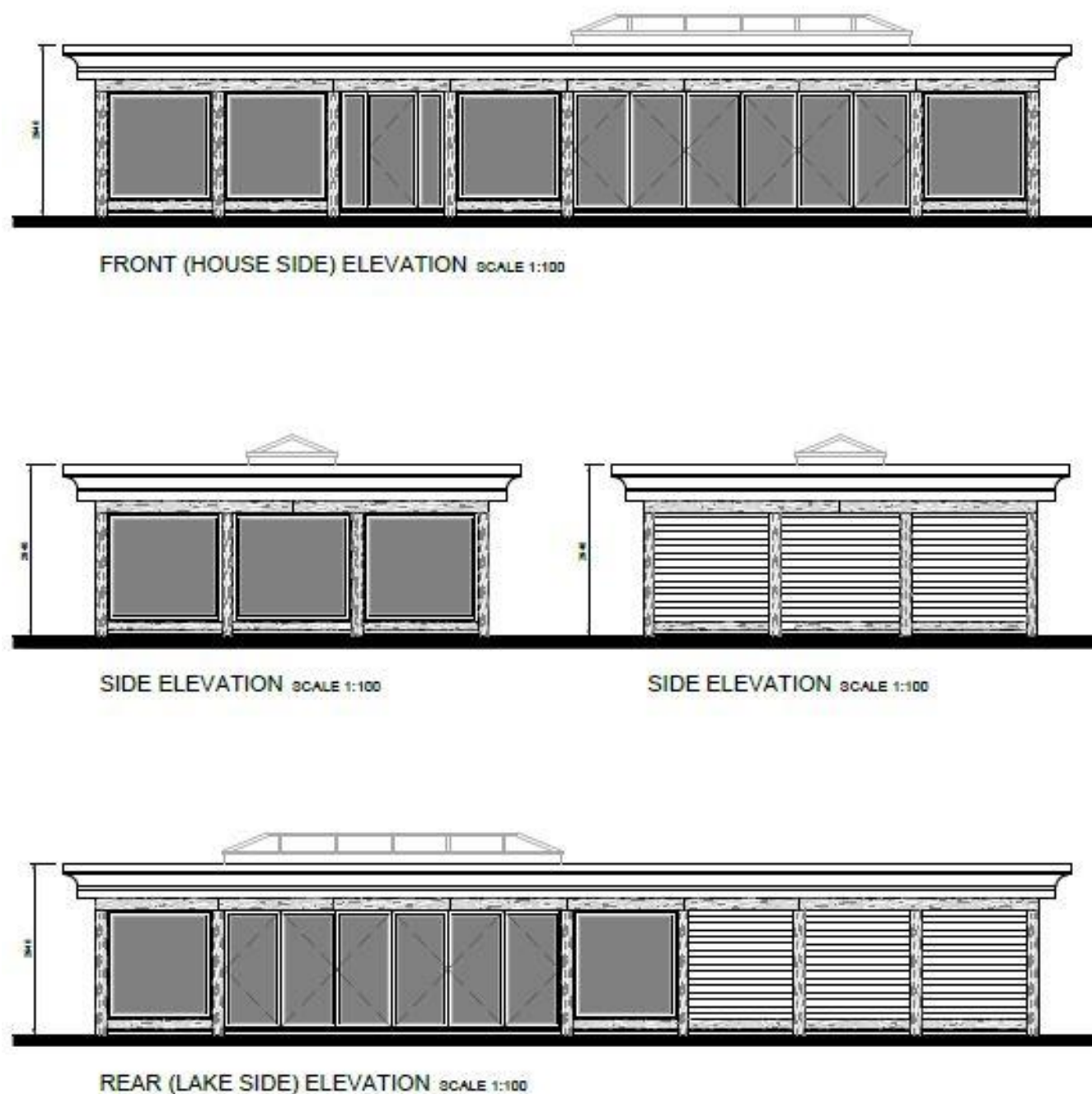
Fig. 27 Lake Side Garden Swimming Pool Outbuilding - Elevations
