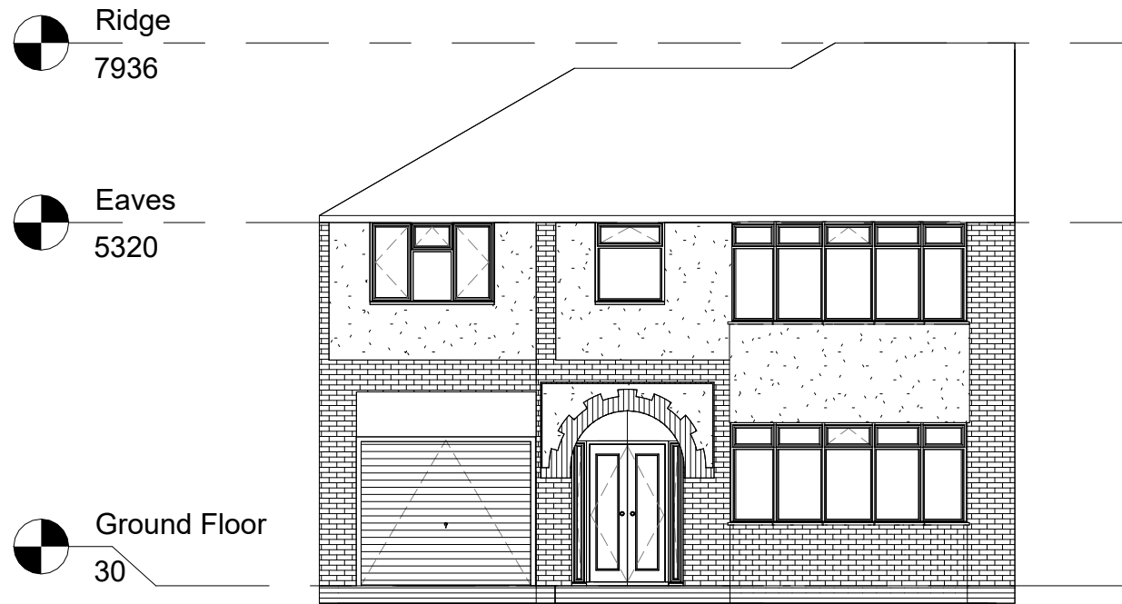
2 Existing Front Elevation 1 : 100
