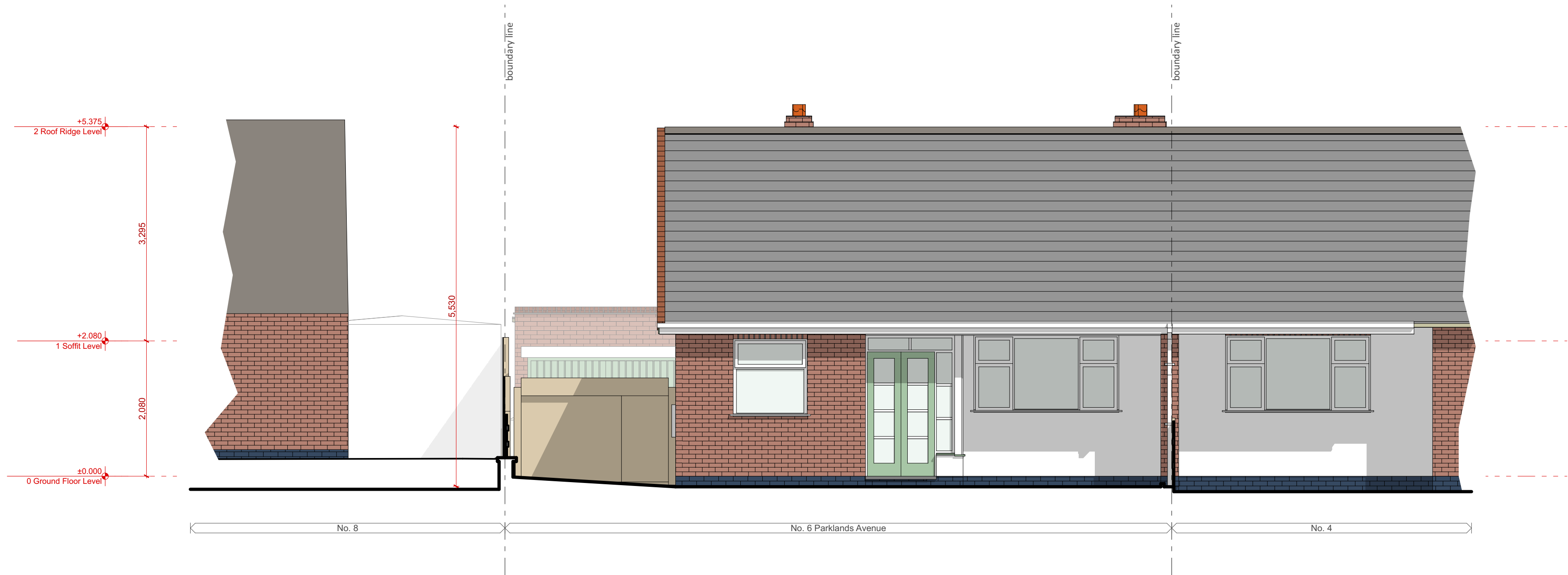
ID: E-01 Existing Front Elevation 1:50
