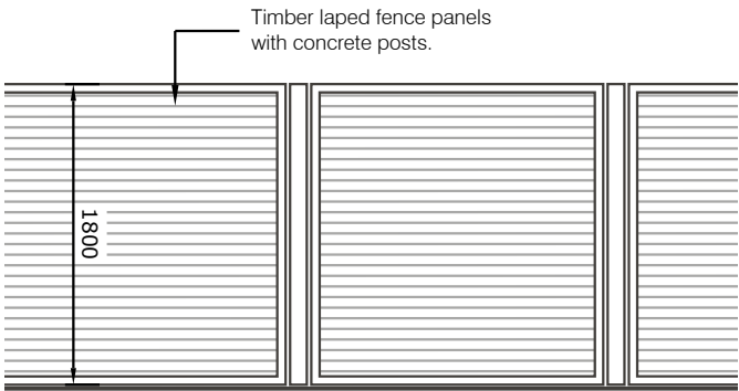
EXISTING BOUNDARY FENCE scale 1:50
