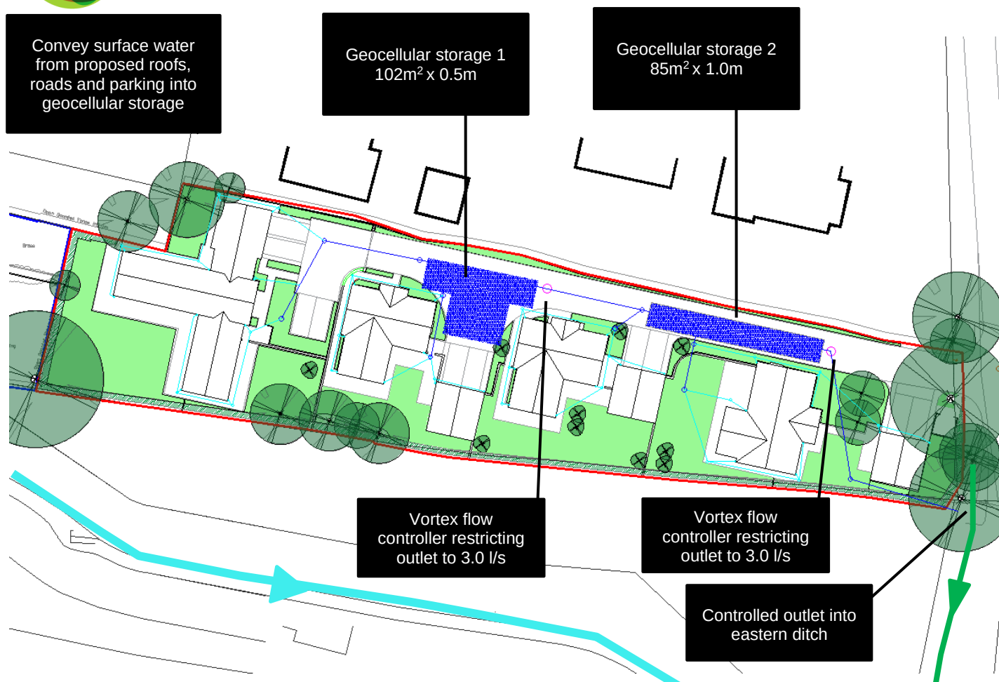
FIGURE 3: PLAN SHOWING THE CONCEPTUAL SURFACE WATER DRAINAGE SCHEME
