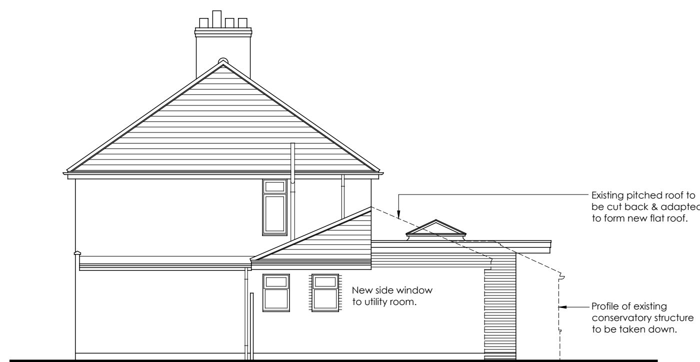
SIDE ELEVATION NORTH
