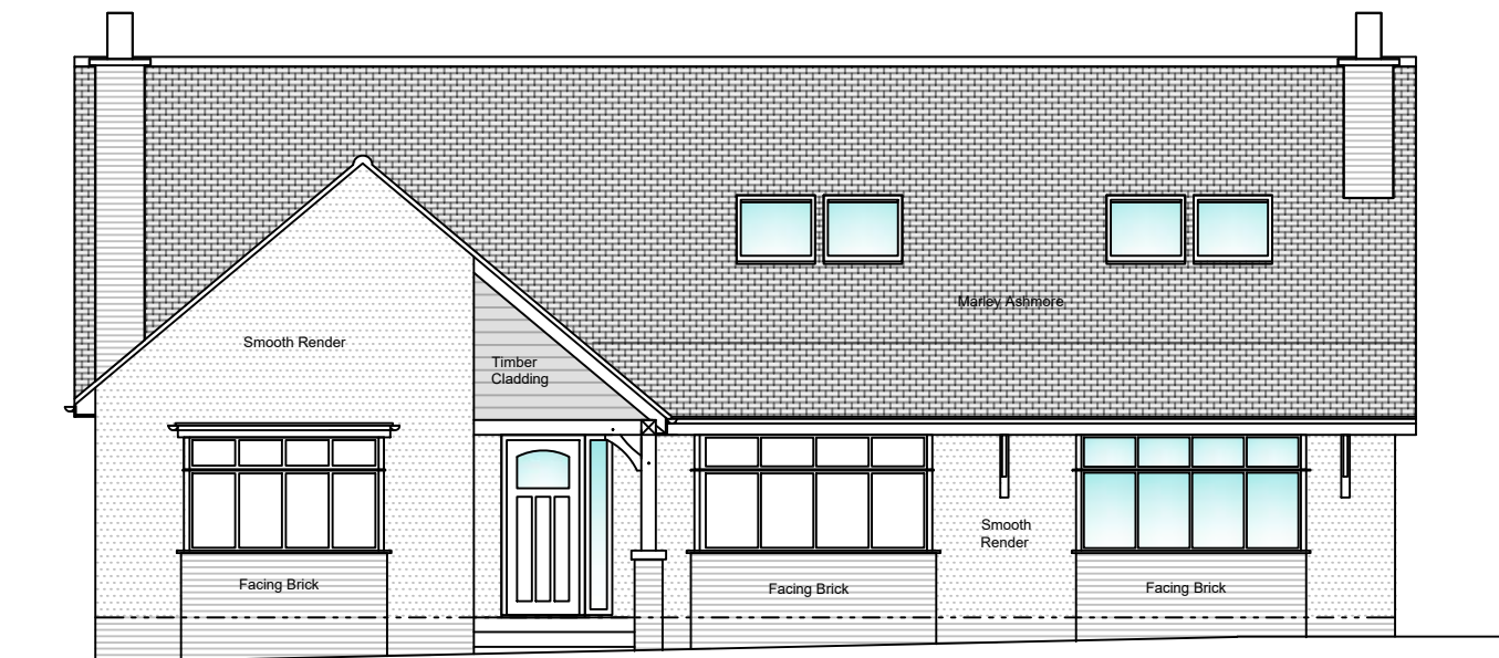
Prop. North - West Elevation
