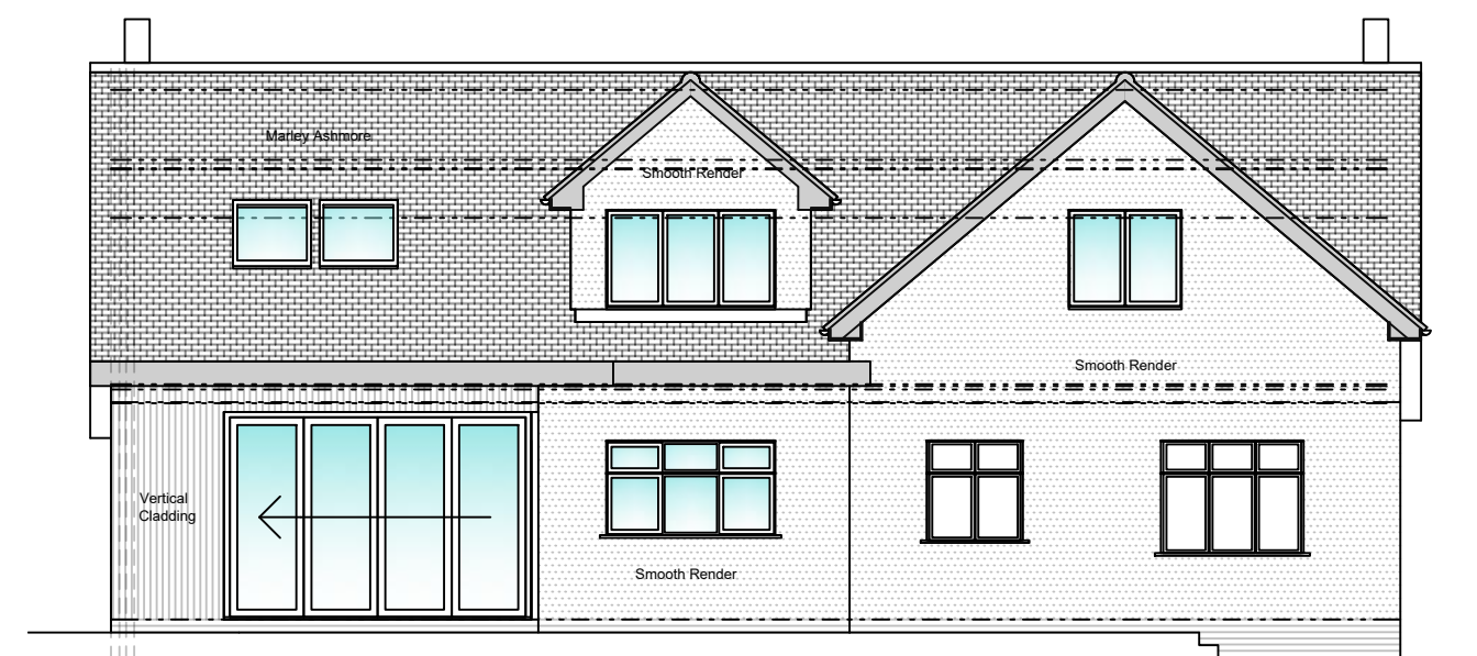
Prop. South - East Elevation
