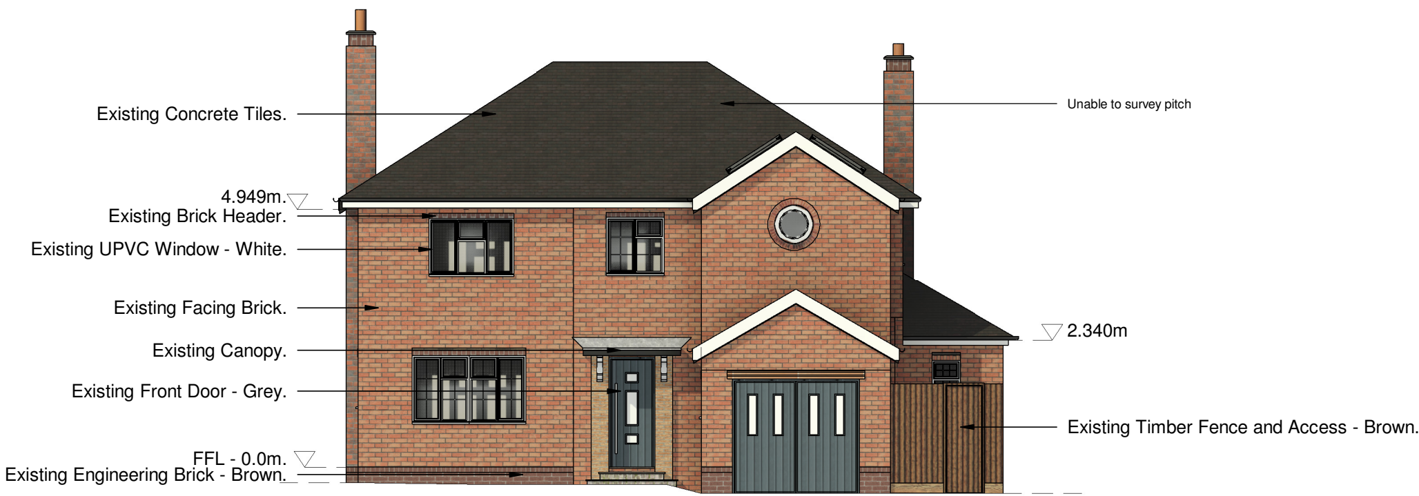
Front Elevation Scale @ 1:100
