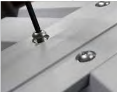
Step 1 Undo the LED chevron from the luminaire spine
