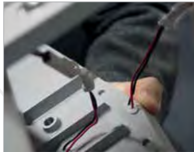
Step 3 Remove the old LED chevron
