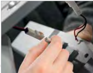
Step 2 Disconnect the old LED chevron using the 'plug & play' connectors
