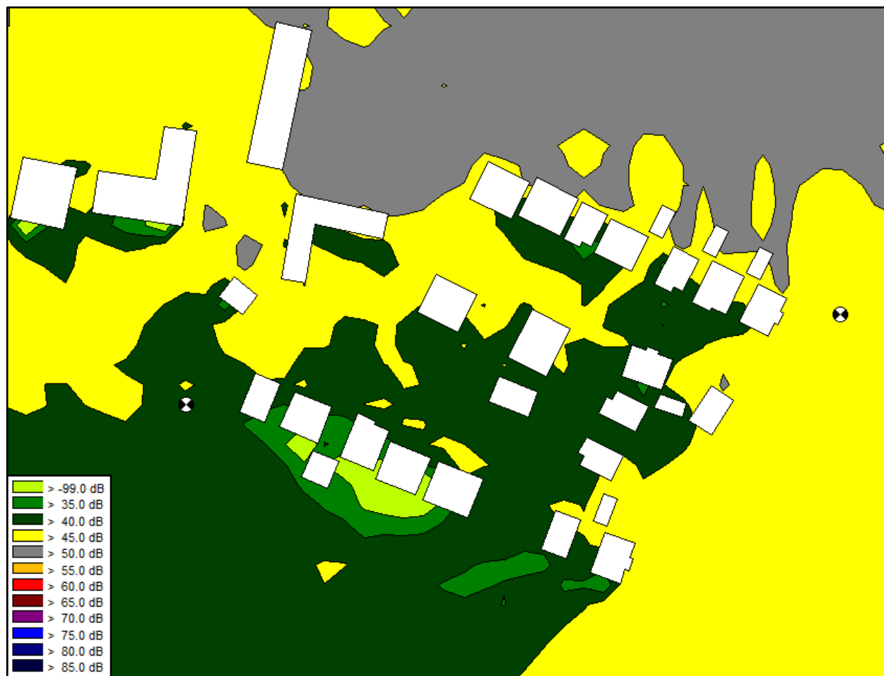
Figure 4: Plan view of the CadnaA model – Daytime L_{Aeq,16hr} (dB) noise levels at 4.5 m
