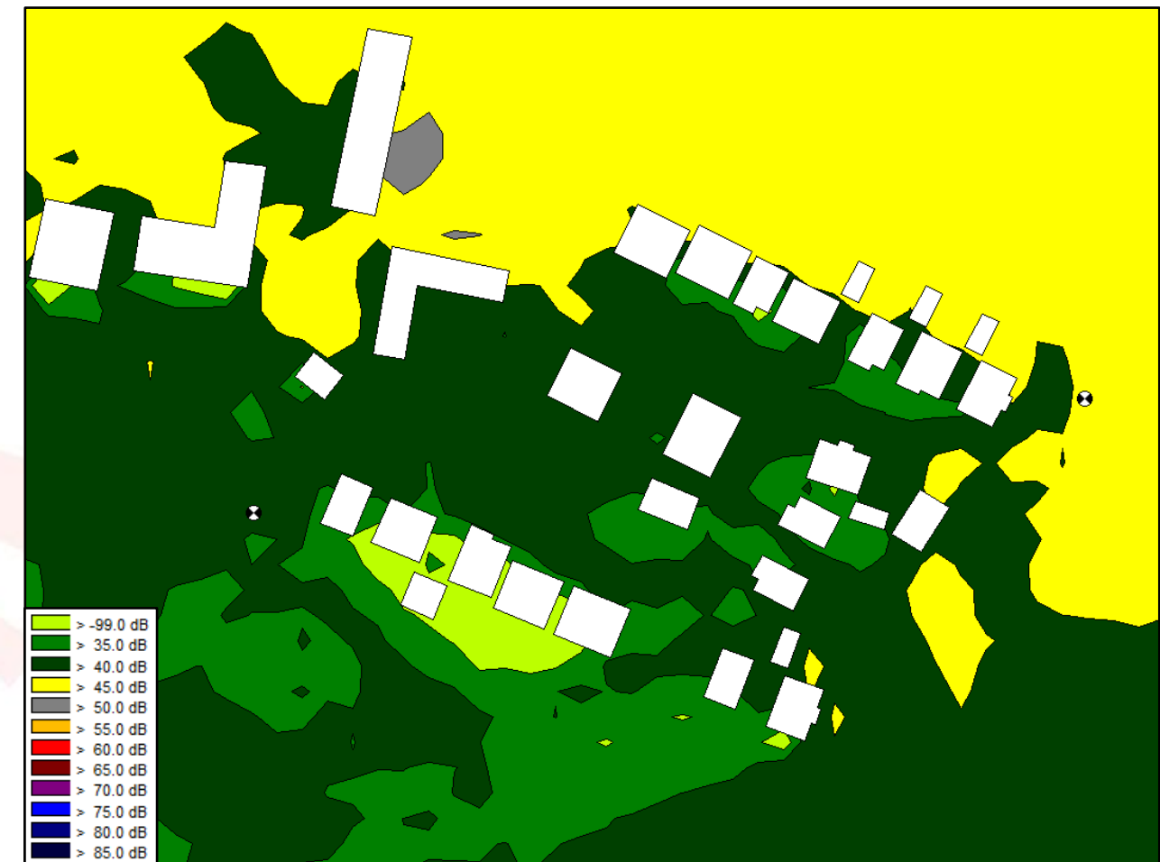
Figure 5: Plan view of the CadnaA model – Night-time L_{Aeq,8hr} (dB) noise levels at 4.5 m
