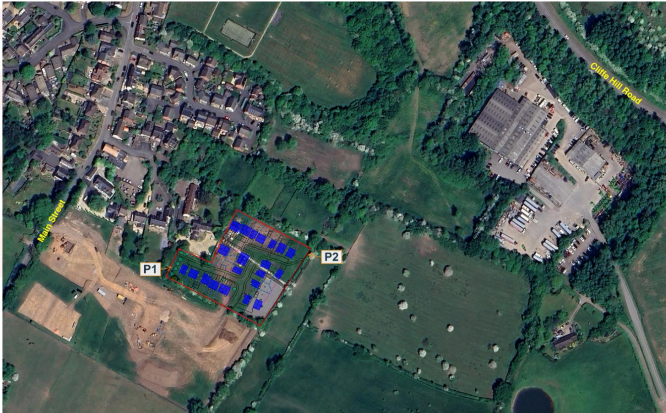
Figure 3: Development site boundary (red), new houses (blue) and noise survey measurement positions (orange)
