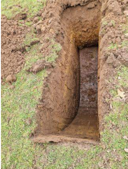
PLATE 13 – Trial Pit Excavation – TP04.
