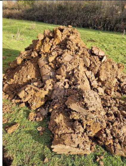
PLATE 22 – Trial Pit Spoil – TP08.
