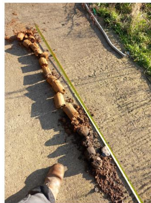
Photo No.6: WS03 full run showing made ground materials (bottom of photo) leading into natural deposits (top)
