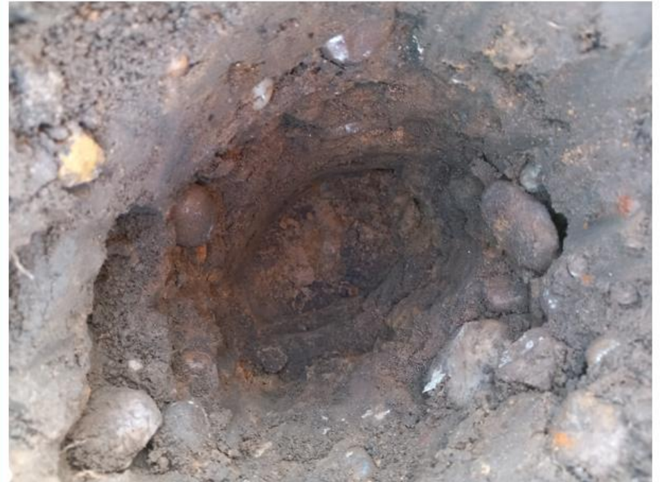
Photo No.12: HP01 pit sides and base showing natural, mixed lithology gravels held in a sandy, clayey matrix
