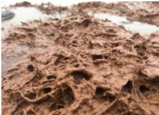
Close up FlocMat showing accretion of silt
