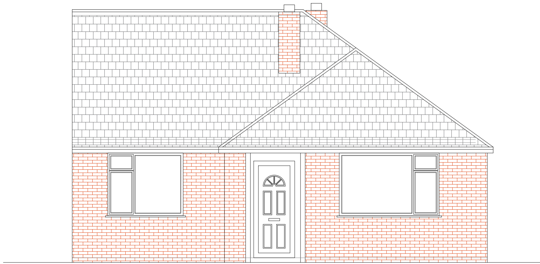
Existing Front Elevation 1:50
