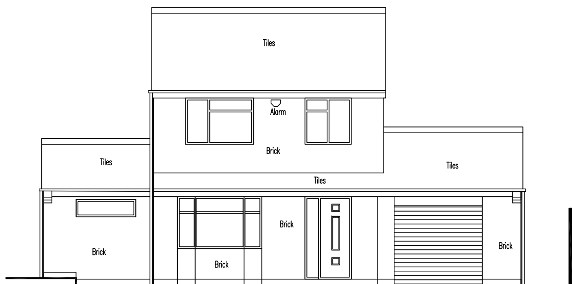
Existing Front Elevation
