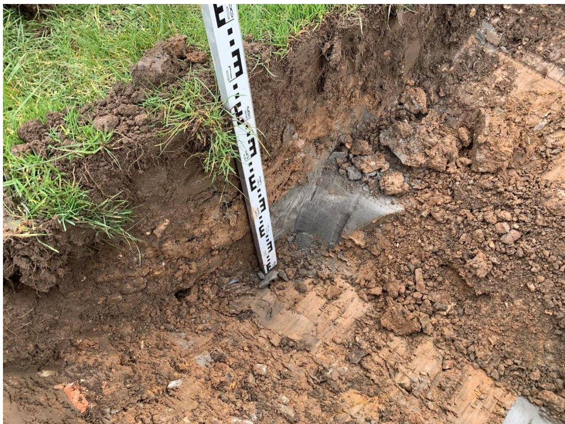
Fig. 19 - Pitch 5 area topsoil and subsoil profile; heavy clay, waterlogged surface, building rubble buried in the eastern strip
