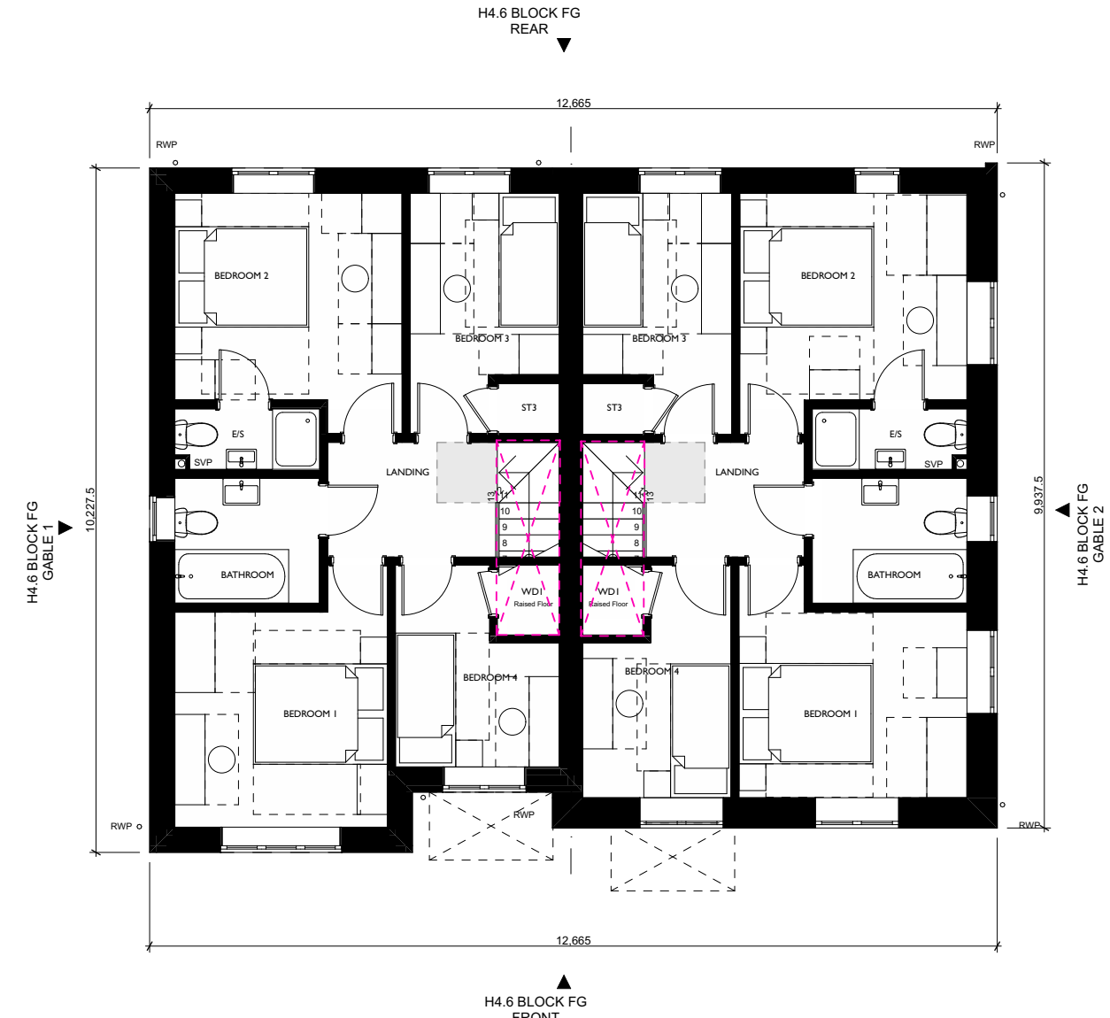
BLOCK FG FIRST FLOOR 1:100
