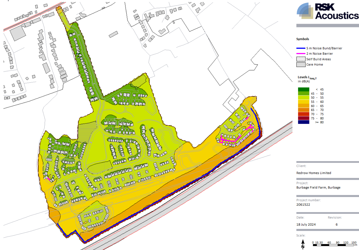
Figure 5 Night-time Ambient Noise Levels L_{Aeq,8h} .
