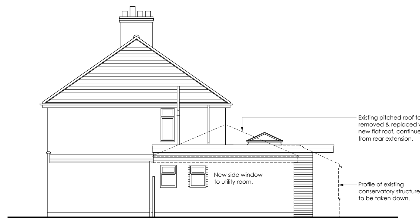
SIDE ELEVATION NORTH
