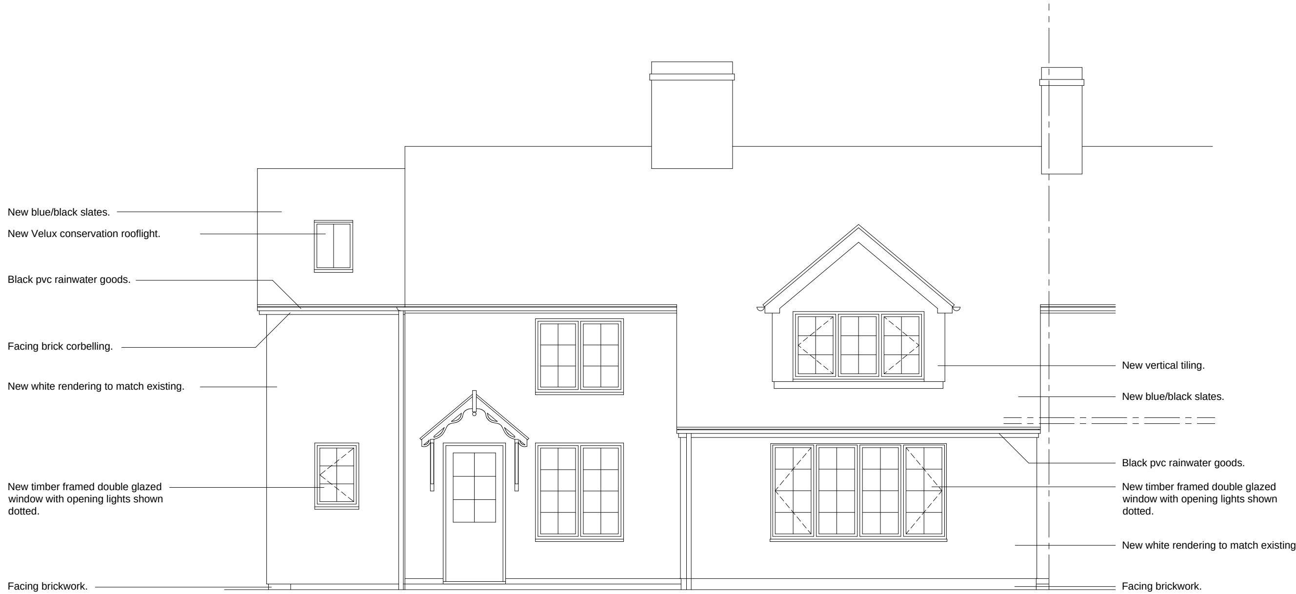
PROPOSED FRONT ELEVATION (South East)
