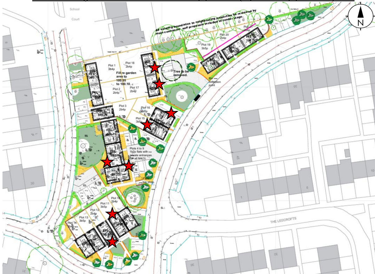
Figure 8: Annotated site plans to show the locations of the of the integrated bat boxes to mitigate for the loss of common pipistrelle ( Pipistrellus pipistrellus ) bats
