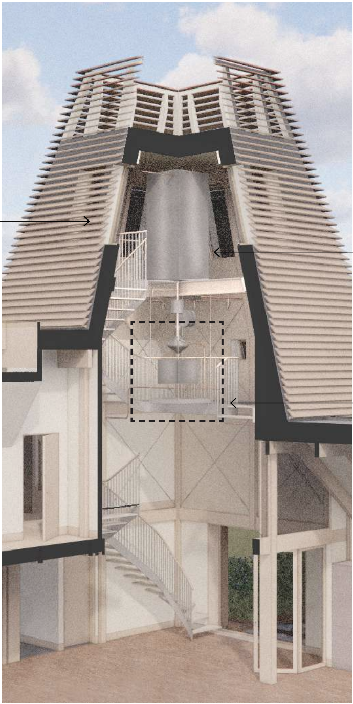
Water Tower: perspective section
