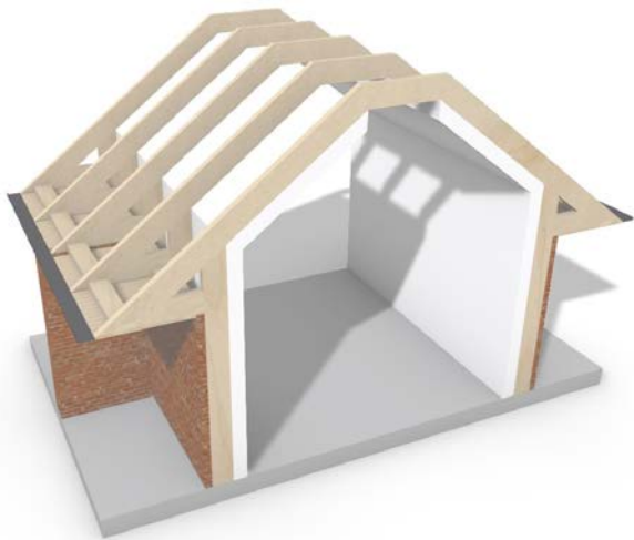
OPTION 4 - BUTTRESSES WITH EXTERIOR 'COLD STRUCTURE'
