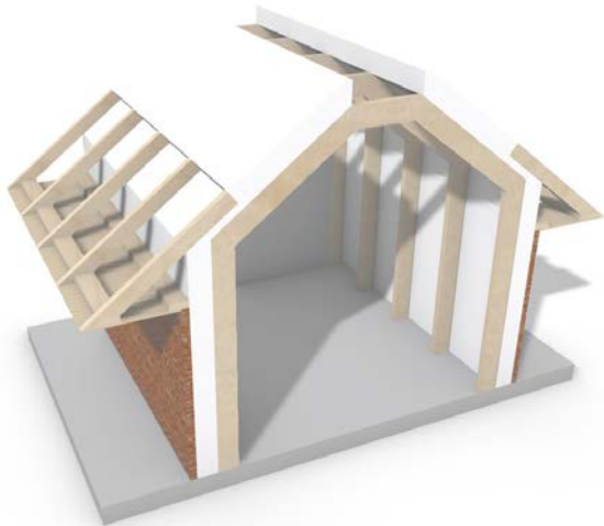
OPTION 1 - SHEAR WALLS AS SPECIFIED BY ENGINEER
