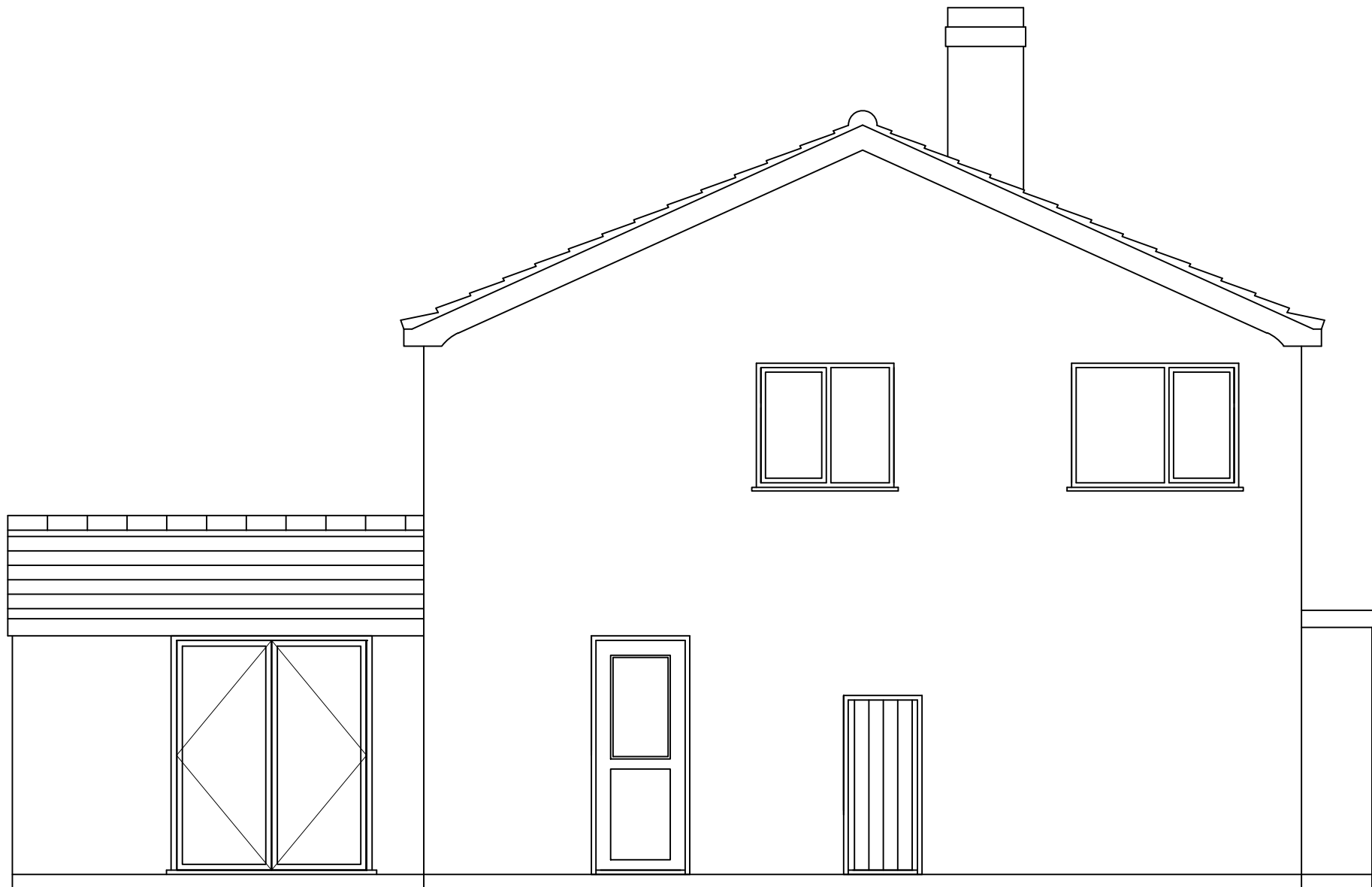
Existing Gable Elevation Scale 1:50
