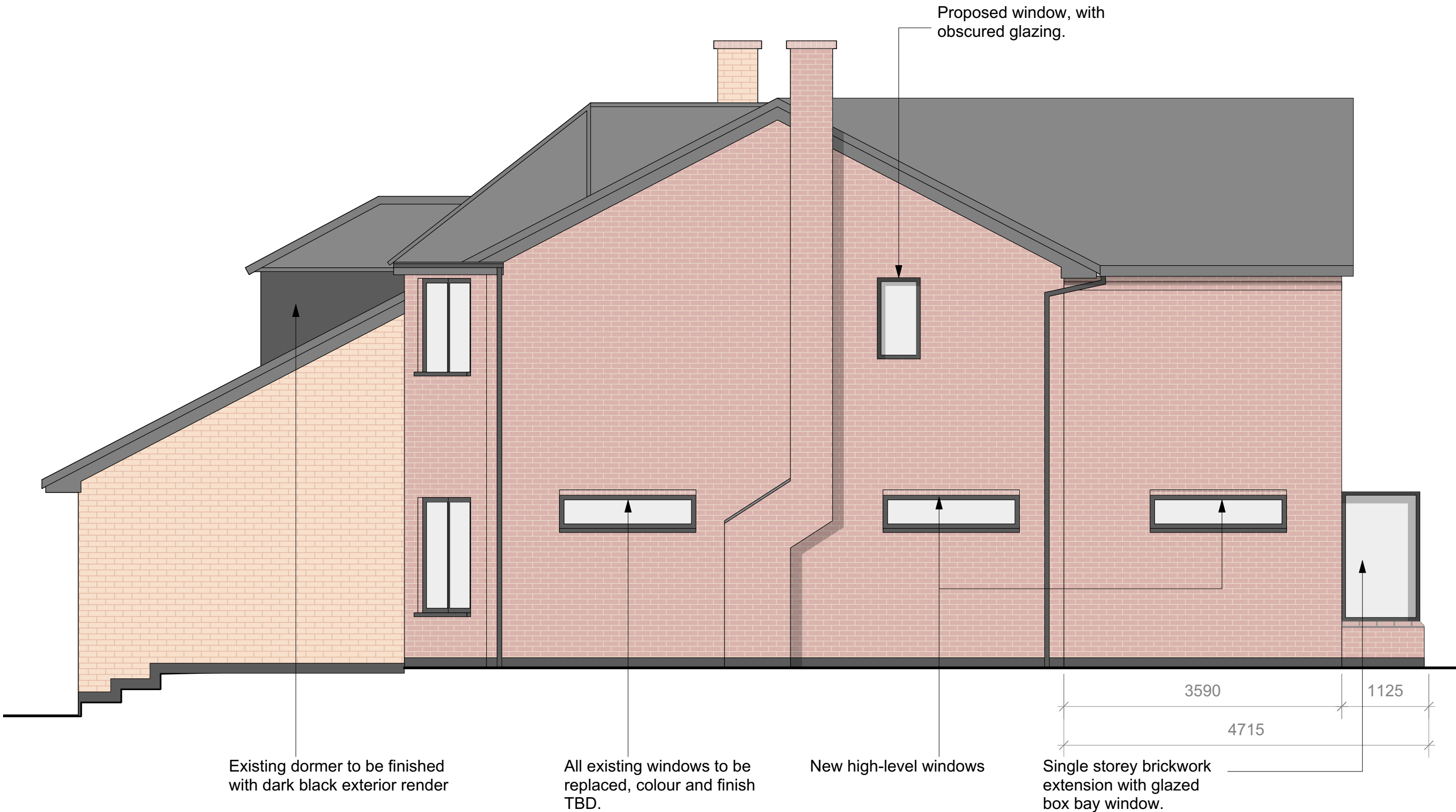
East Elevation (Side)
