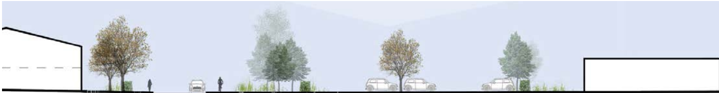
Indicative Section | 7-9m | 2m | 7.3m | 3m | 12m | 6m | 4.8m | 4.8m | 6m | 4.8m | 9m | 18m
