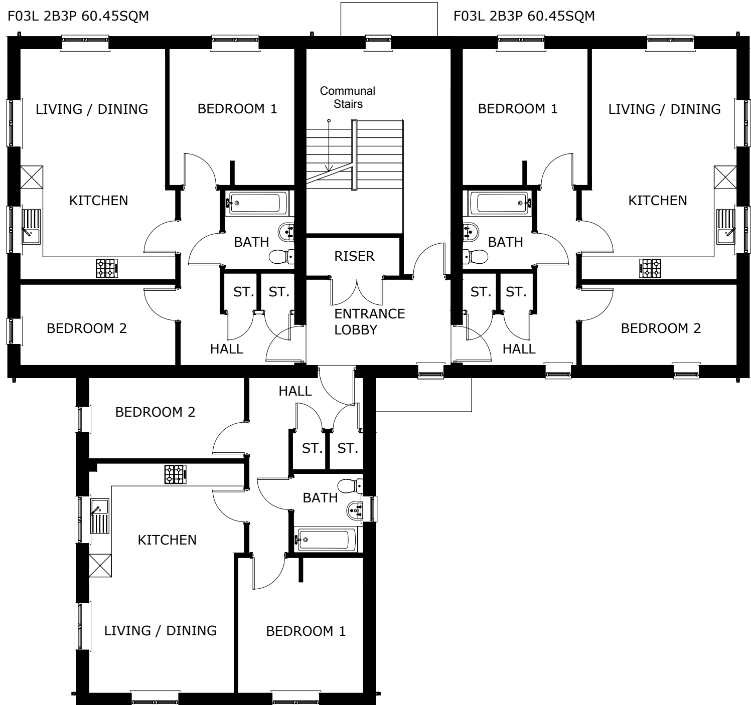
F03L 2B3P 60.27SQM FIRST FLOOR PLAN
