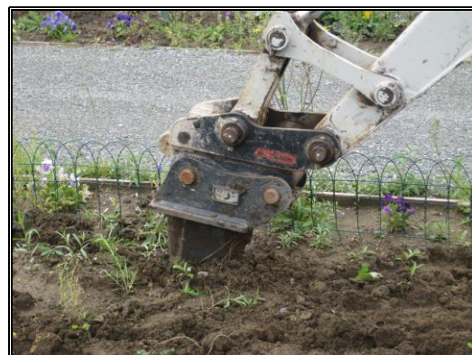
Plate 4 : Single rigid tine in use
