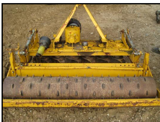
Plate 5: Example of power harrow
