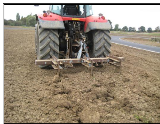
Plate 2 : Tractor drawn subsoiler
