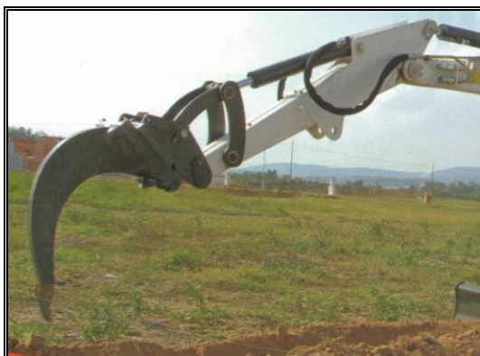
Plate 3: Tracked excavator with single rigid tine
