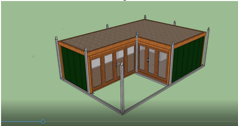
Vertical sections fitted at key points around structure with lifting points visible.
