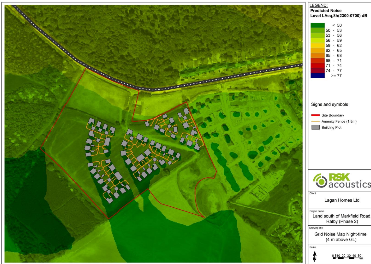
Figure C.2 Night-time noise contour map (4m height)
