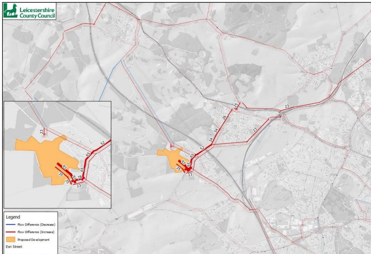
Figure 16. Forecast Flow Change for 2028 PM 'With Development' minus 'Without Development'
