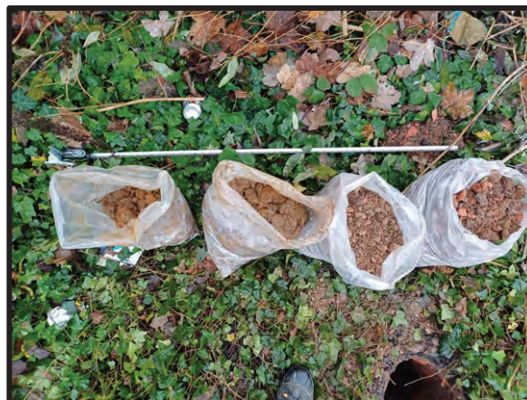
Starter pit arisings
