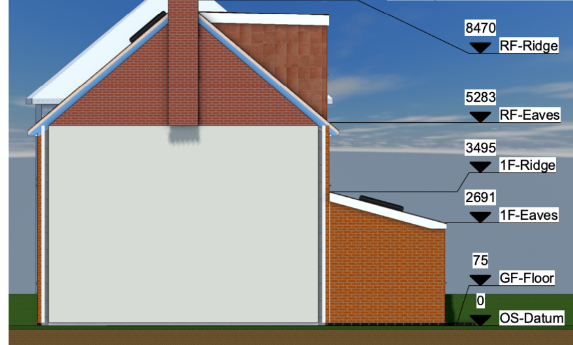
4 South-West Elevation - Proposed Scale: 1:100
