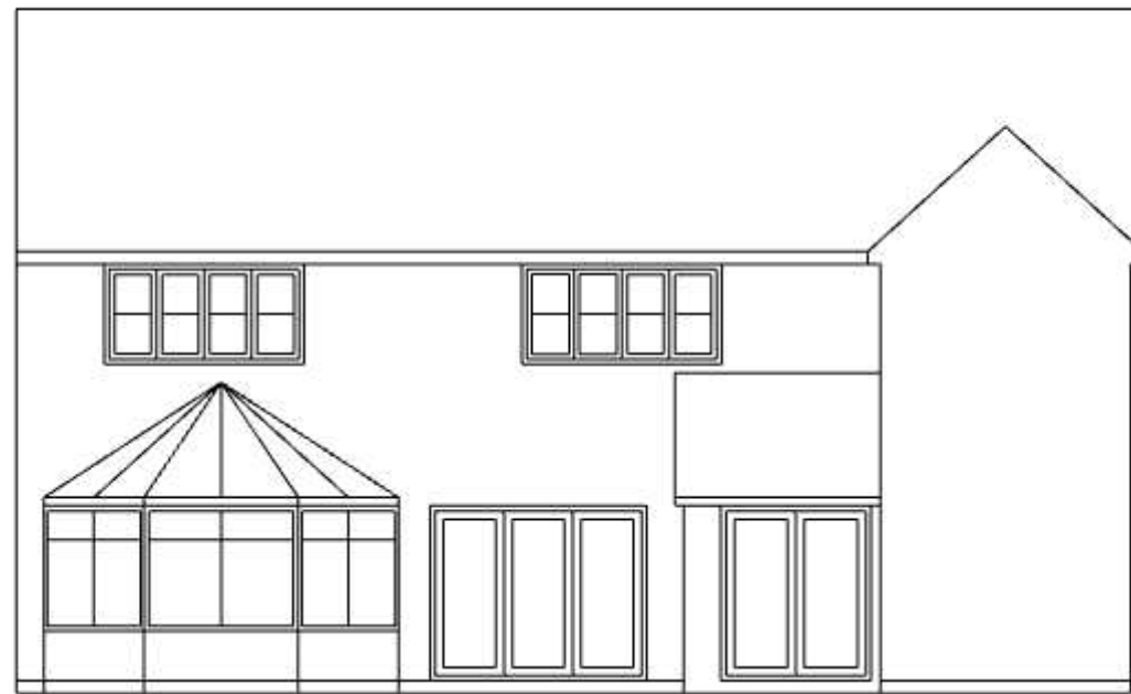
Existing Rear Elevation
