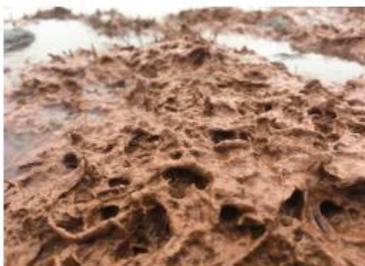
Close up FlocMat showing accretion of silt
