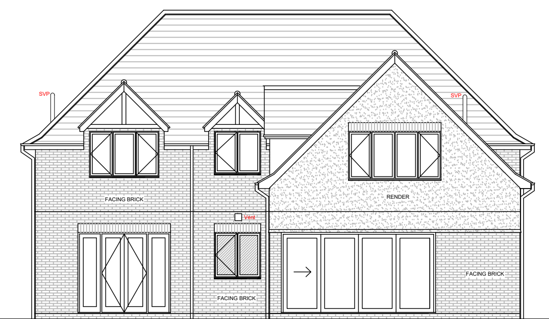
Existing Rear (North) Elevation Scale 1:100
