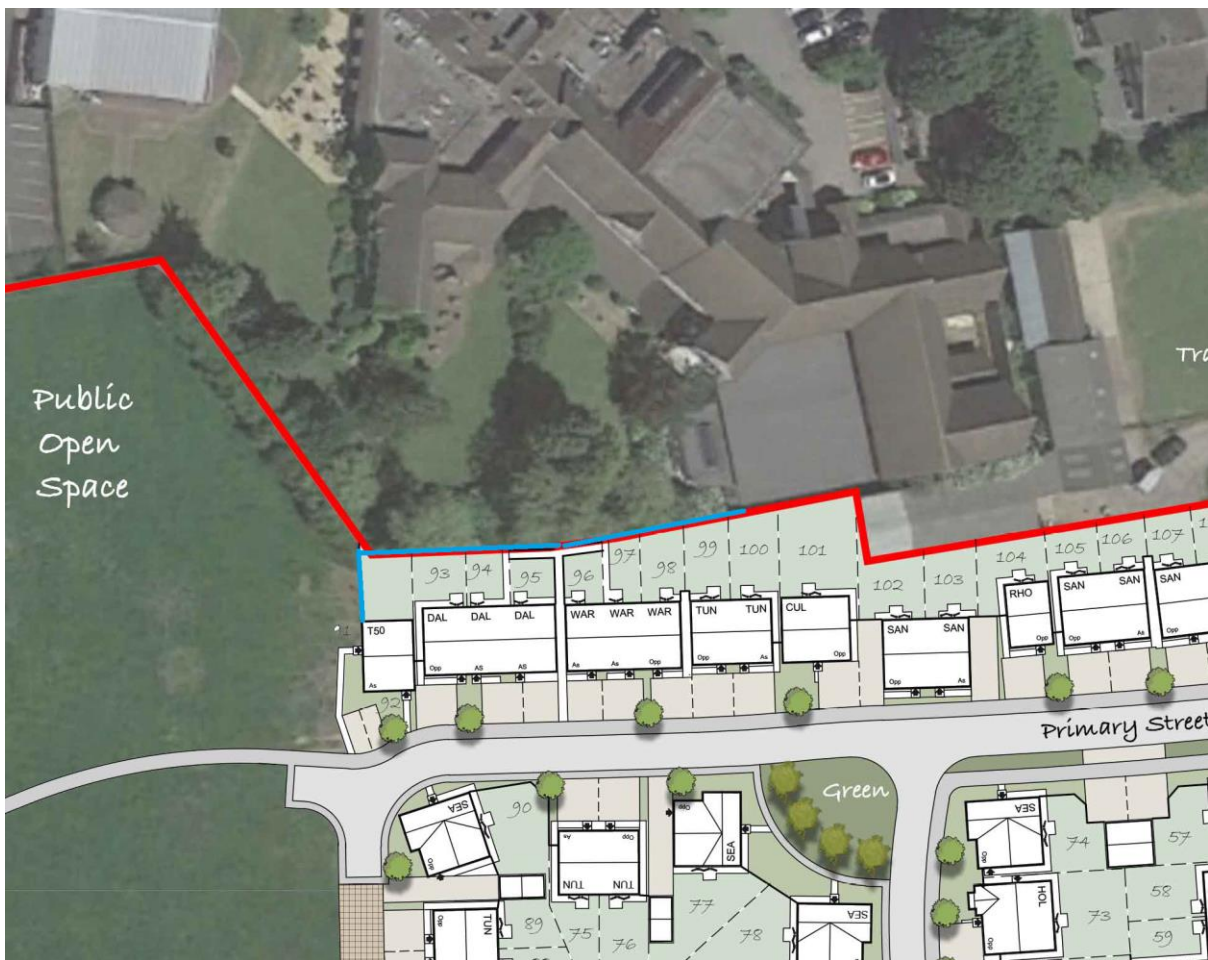
Figure 6 – Acoustic Barrier Location for Hotel
