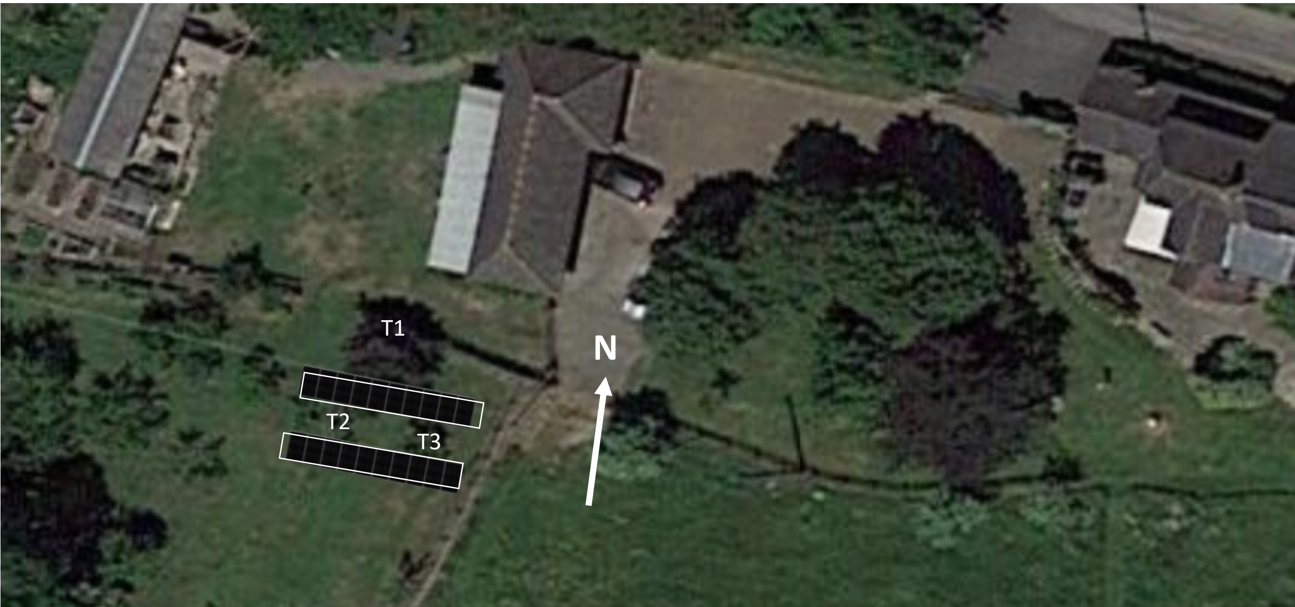
Solar arrays of 10 panels (each 1m wide x 2m high) two boxes outlined in white
