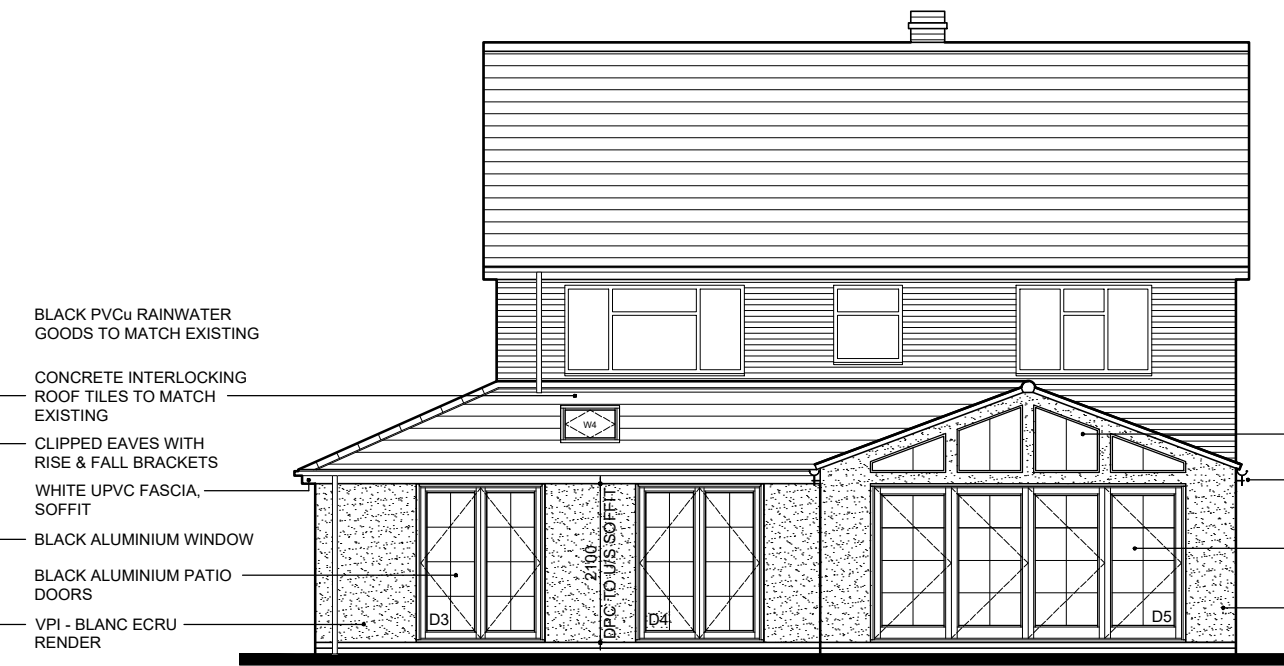
REAR (NORTH) ELEVATION
