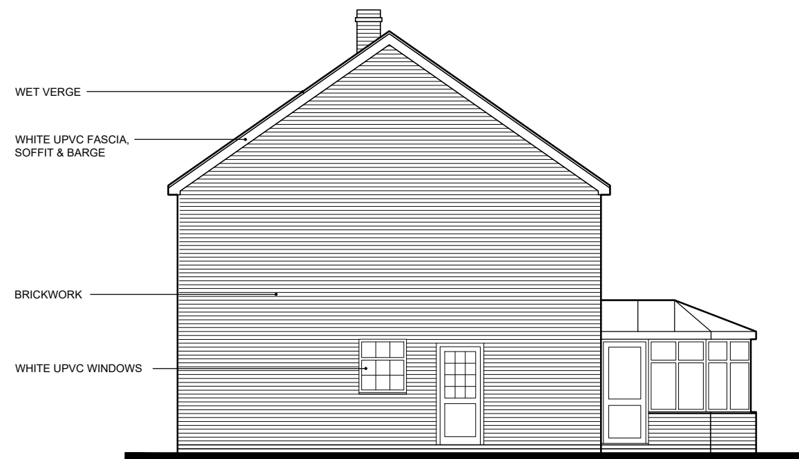
SIDE (EAST) ELEVATION
