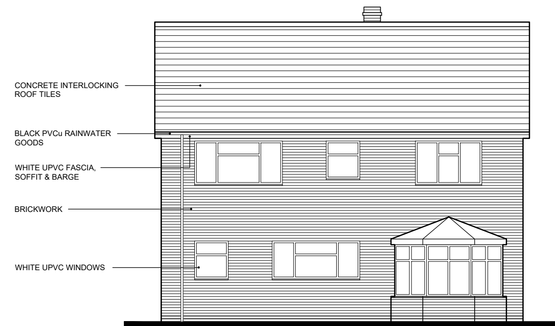
REAR (NORTH) ELEVATION
