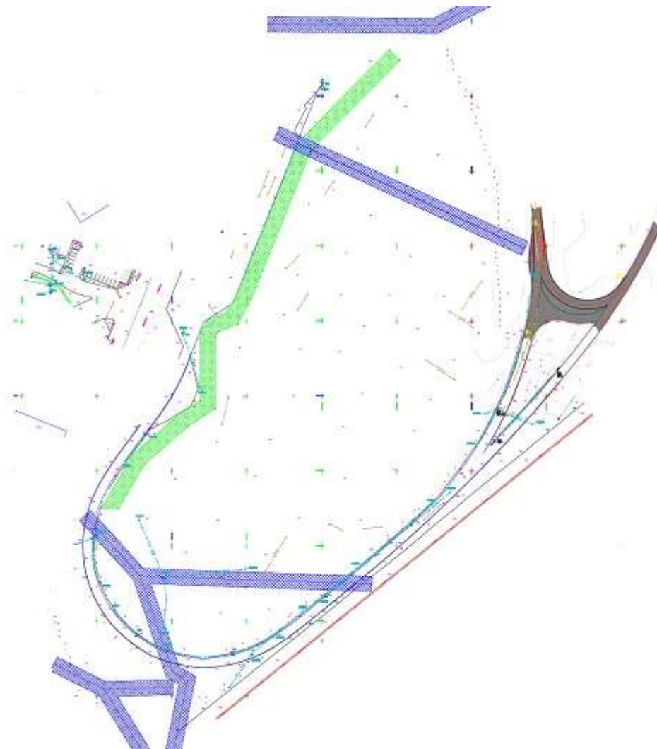
Figure 2: Detailed site location plan showing known underground services (blue and green lines) (provided by client).
