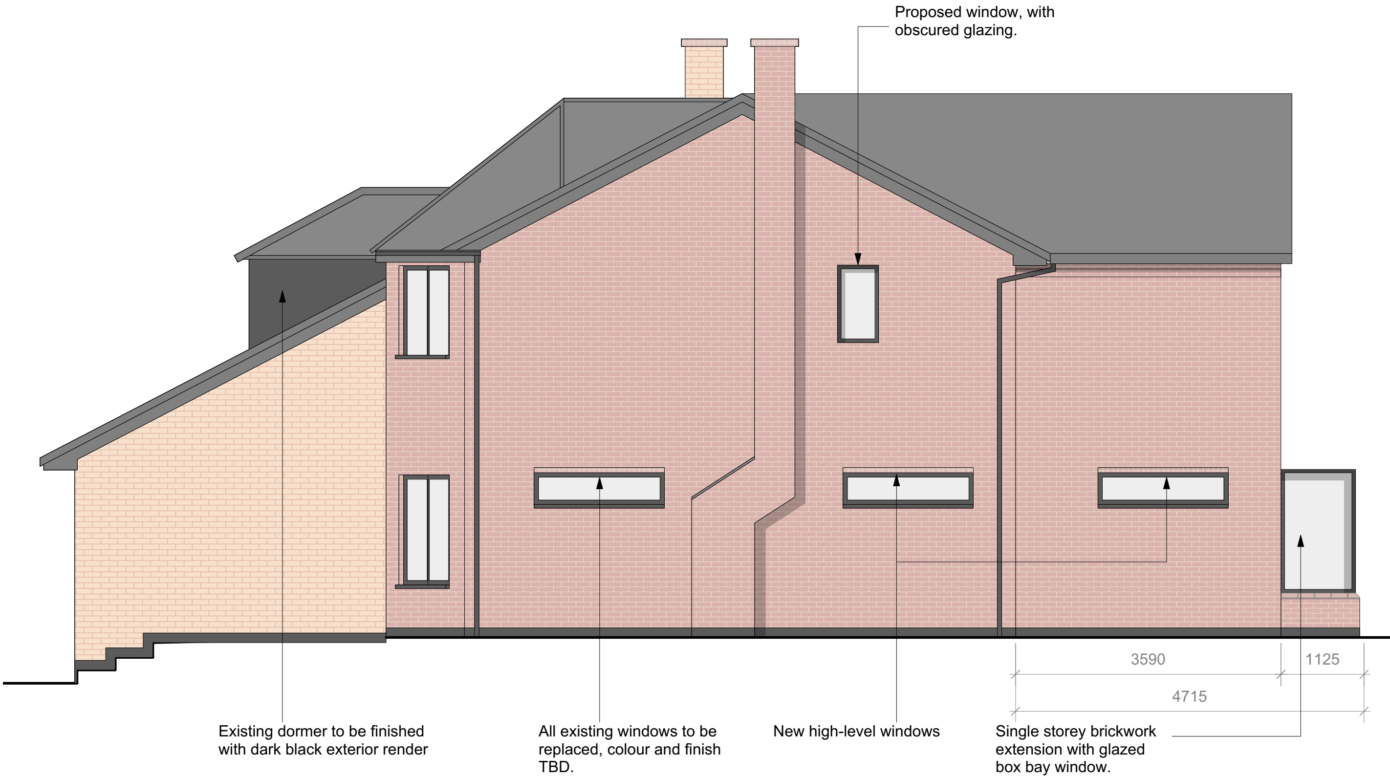
East Elevation (Side)
