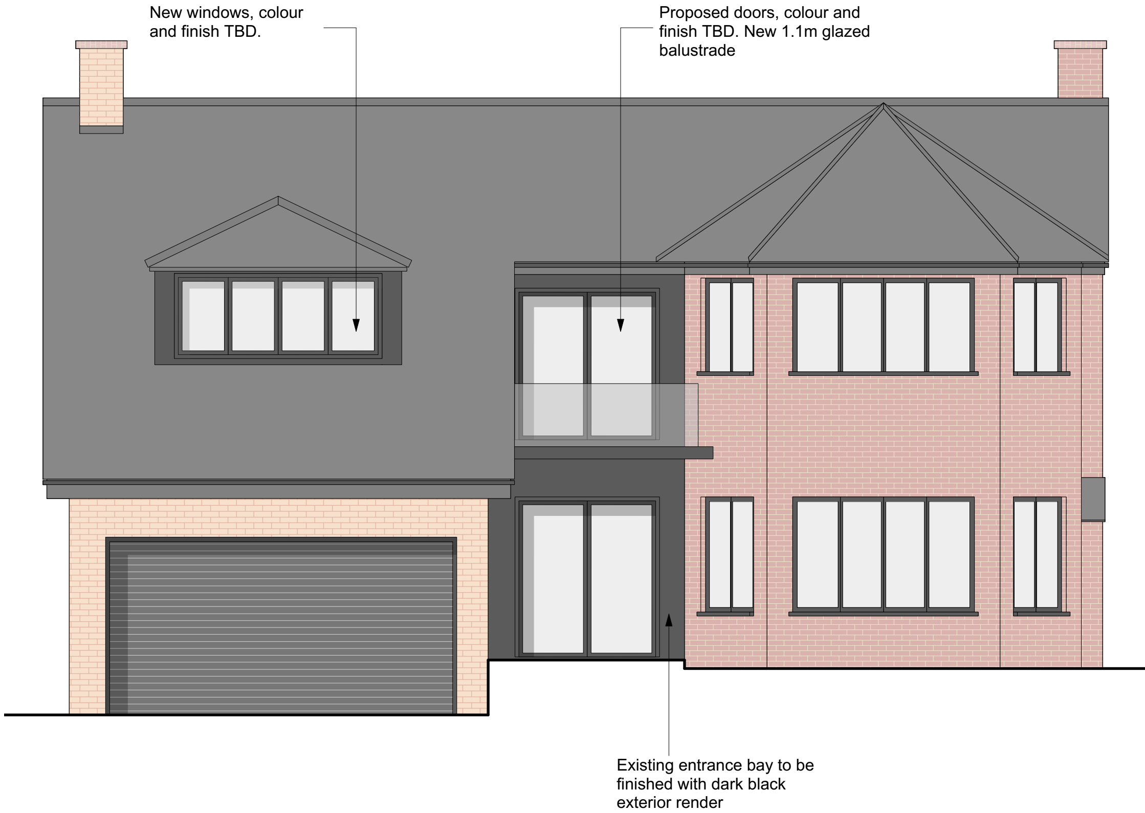
North Elevation (Front)
