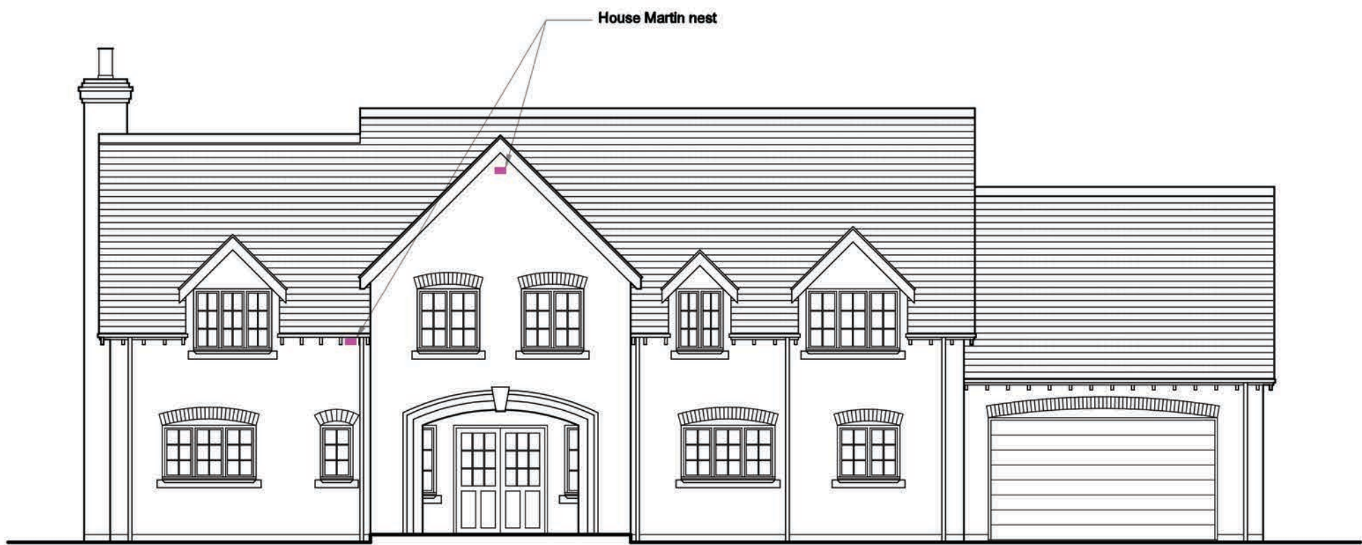
ELEVATION - facing north. Scale 1/100.
