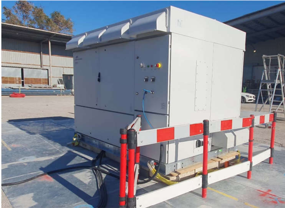
Illustration 5. Views of the PCSK Gen3 inverter without acoustic attenuation kit
