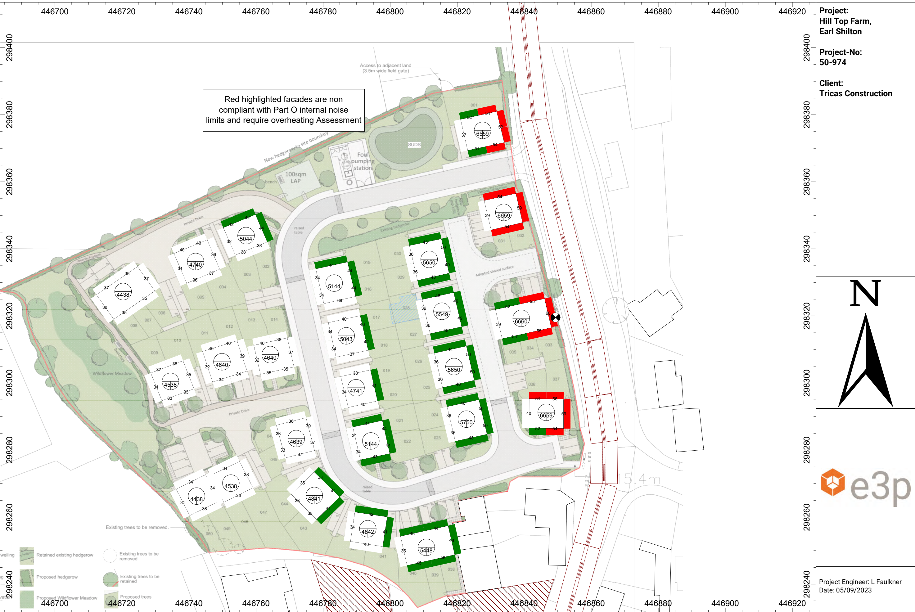
Figure 5 - Part O Overheating Requirements
