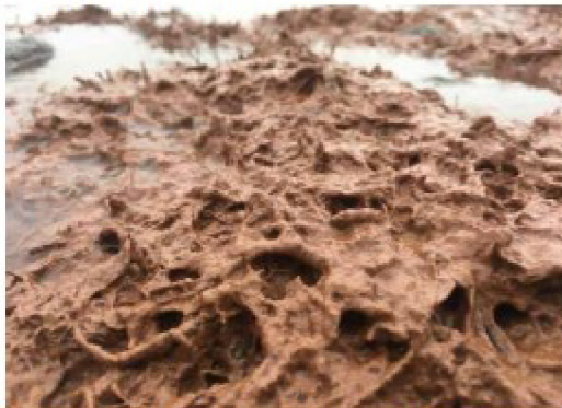
Close up FlocMat showing accretion of silt
