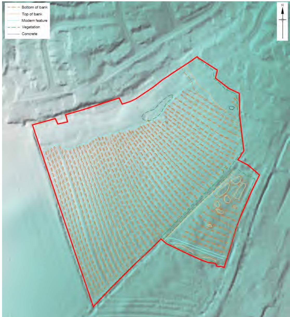
Plate 13 Results of the earthwork survey
