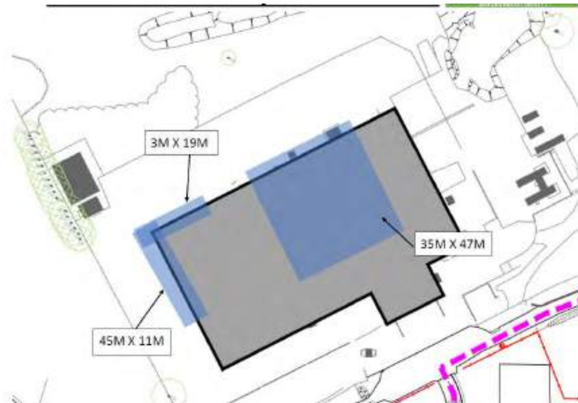
Figure 1 – Approximate Locations of ACMs under building footprint
