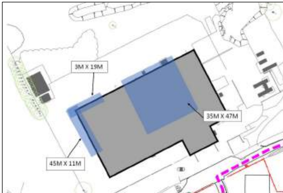
Figure 4-1 Location of ACMs under Building 1 footprint
