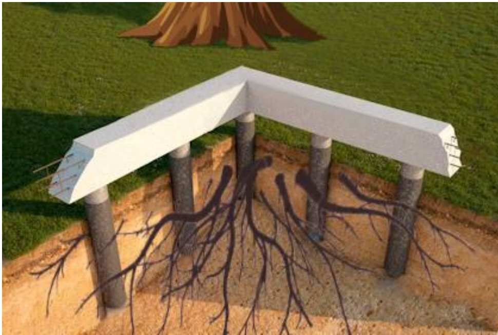
Pile and beam foundations.
