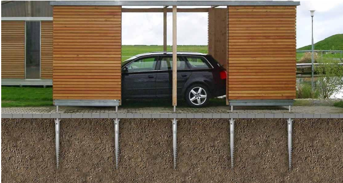
Screw pile foundations.
